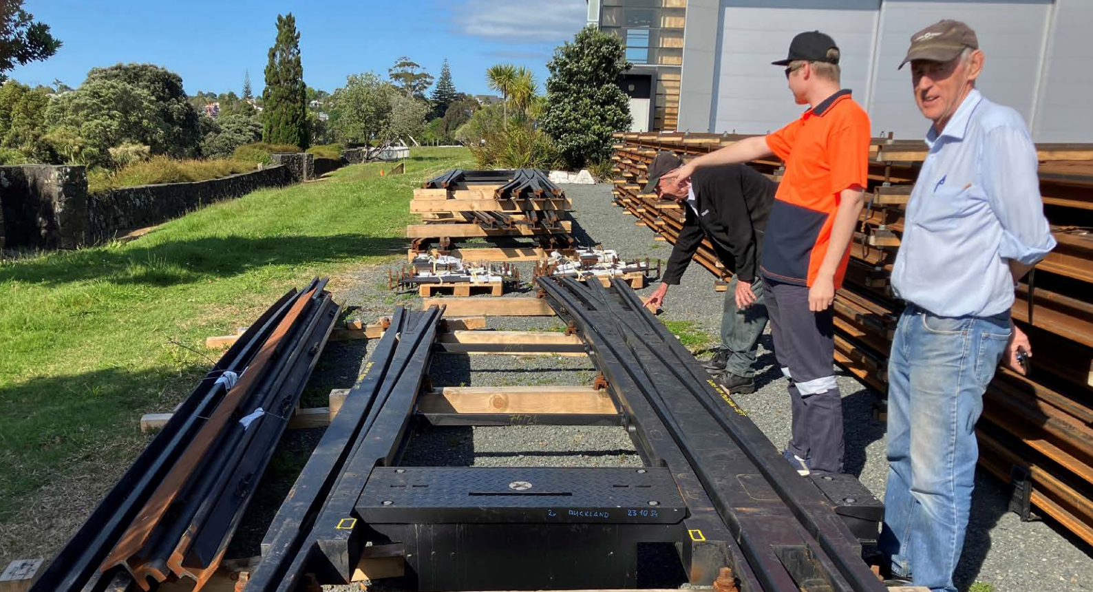
Tony Messenger, Joshua Garratt & John Miller inspect the two new dual gauge point sets. Photo: James Duncan
