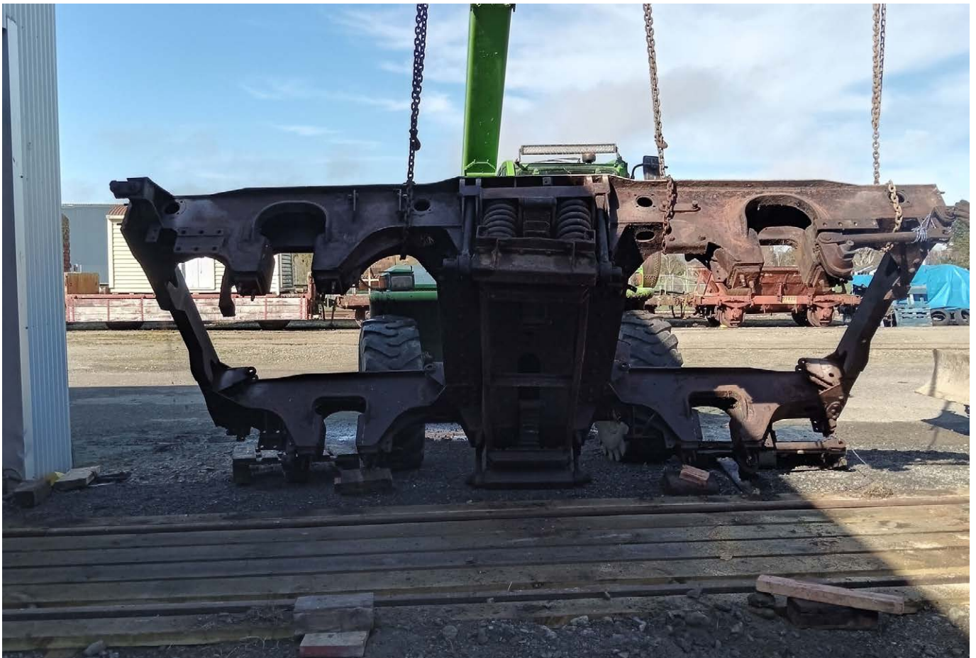
↓ The articulated bogie being flipped and stripped.
